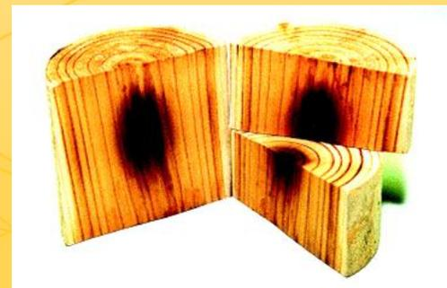
*d. Pyrolysis front development with microwave heating*
