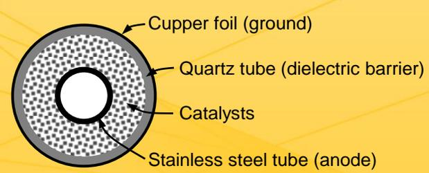
Cross section of the NTP reactor
