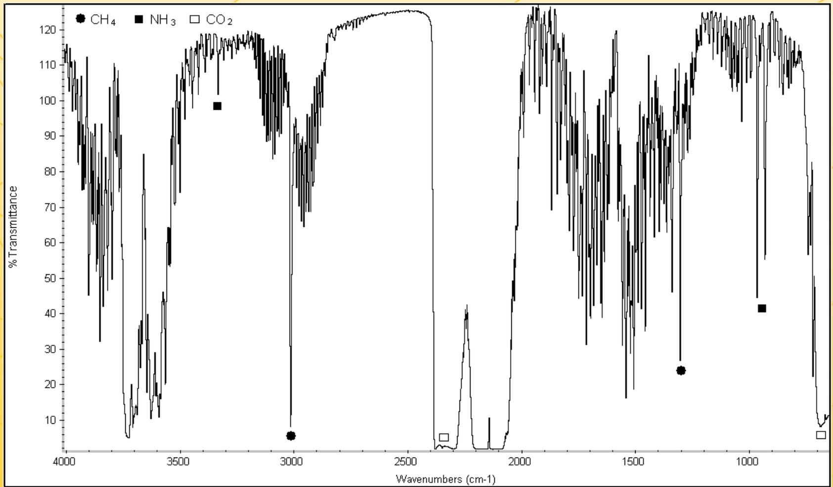
FT-IR spectrum of NTP reforming of N<sub>2</sub>, CO, H<sub>2</sub> and/or H<sub>2</sub>O vapor.
