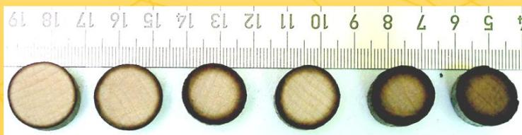
*c. Pyrolysis front development with conventional heating*
