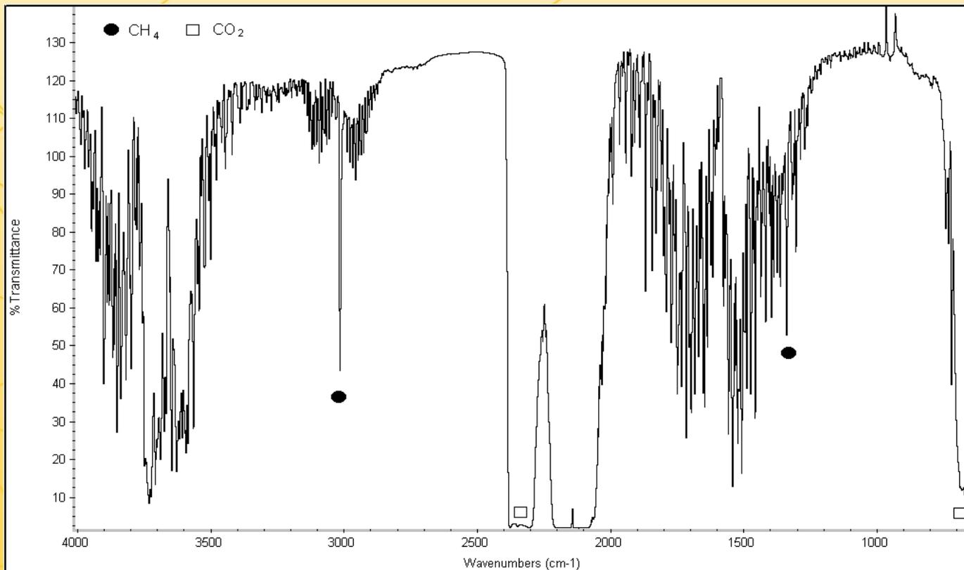
FT-IR spectroscopy of NTP reforming of CO and H<sub>2</sub>O vapor.
