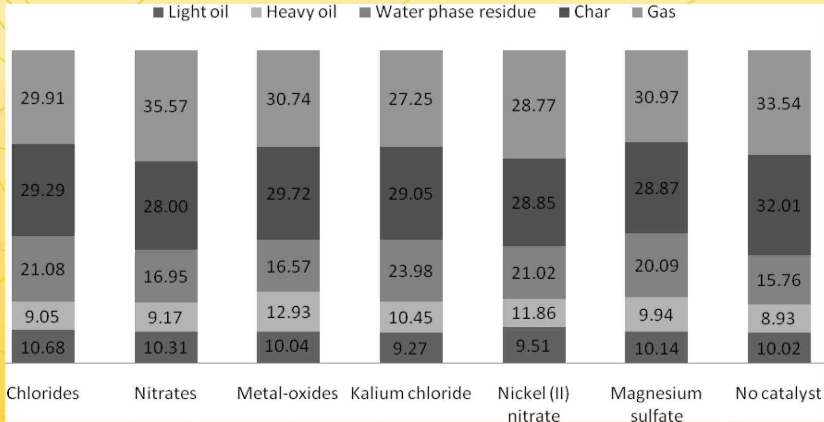
Pyrolysis fraction yields (mass% of total biomass input) from runs with different catalysts and catalyst groups added to the **aspen** pellets
