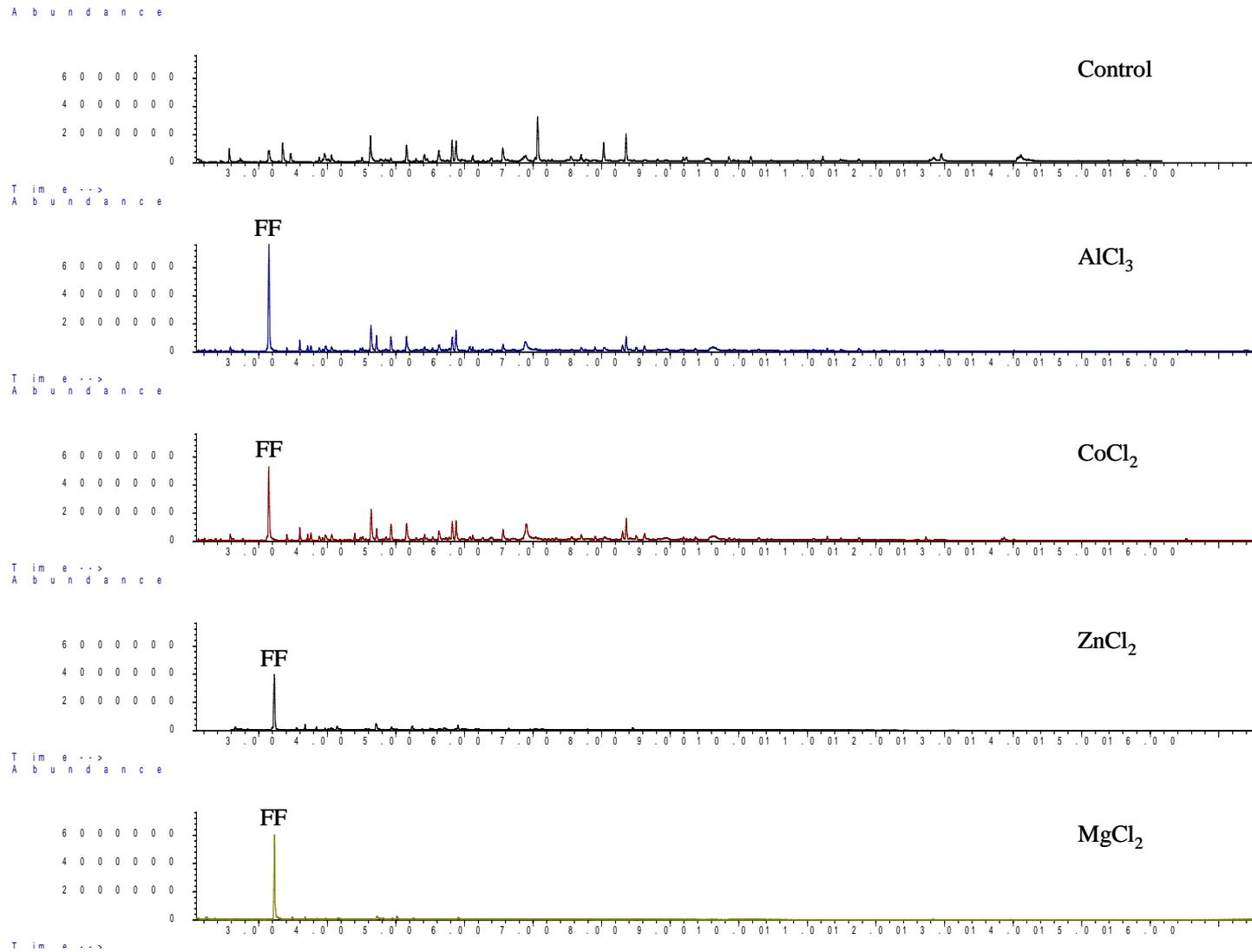
Total ion chromatograms from GC-MS analysis of pyrolytic oils from corn stover when different catalysts were used (8g/100g biomass). FF: furfural.
